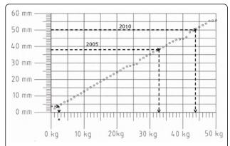
**Figure 1 Force-depth relationship of the manikin used in this study**. Dashed arrows indicate the corresponding force for the minimal recommended chest compression depth of 38 mm (2005 Guidelines), and 50 mm (2010 Guidelines), respectively. The star indicates the threshold used by Fried et al. to define leaning on the patient's chest [20].
